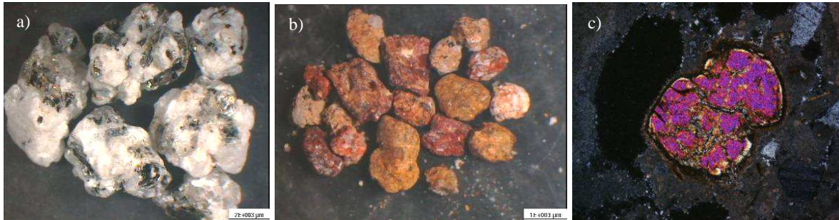
Fig 3. Micrographs of mortars aggregates from Evora's Cathedral a) granitic rock fragments (SEV6), b) ceramic fragments (SEV8) and c) olivine crystal (SEV1) - thin-section (30x).
