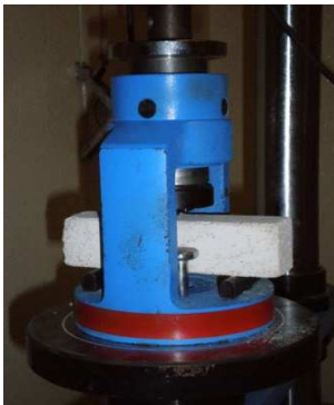
Fig. 3 Equipment used to the determination of specimens flexural and compressive strenght
