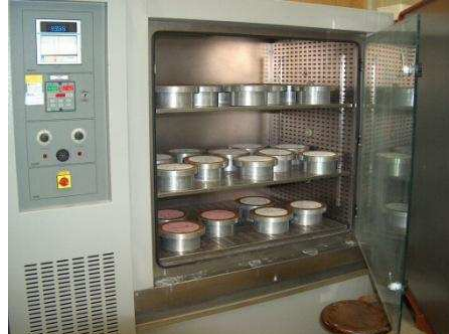
Fig.2 Determination of specimens permeability to water vapour
