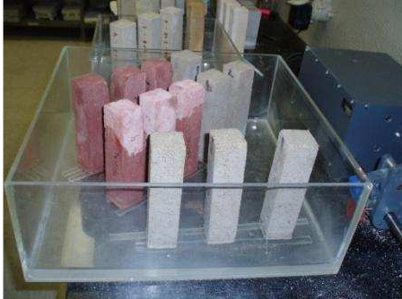
Fig.1 Determination of specimens capillarity absorption
